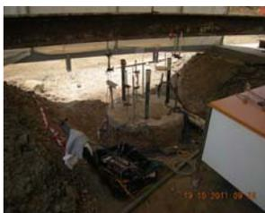
O-Cell Pile test in progress
